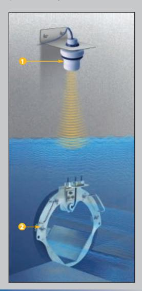
To allow for the monitoring of conditions that change from open channel flow to submerged flow (as experienced in sewers during a storm event or downstream blockage), a maintenance-free, "above the flowstream" independent level sensor can be provided for all Cartridge Meters.
